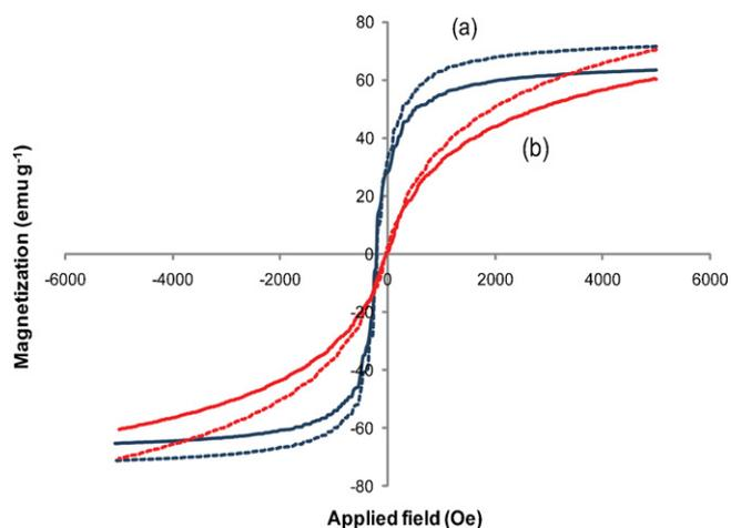
**Fig. 4.** Room temperature magnetization curves of (a) SPIONs (blue) and (b) commercially available MNP (red) before (---) and after (—) conjugated with OVA. (For interpretation of the references to color in this figure legend, the reader is referred to the web version of the article.)
