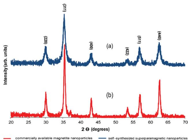
**Fig. 5.** XRD spectra of (a) SPIONs (blue) and (b) commercially available MNP (red). (For interpretation of the references to color in this figure legend, the reader is referred to the web version of the article.)
