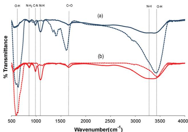
**Fig. 8.** FTIR spectra of (a) SPIONs (blue) and (b) commercially available MNP (red) before (—) and after (---) conjugated with OVA. (For interpretation of the references to color in this figure legend, the reader is referred to the web version of the article.)
