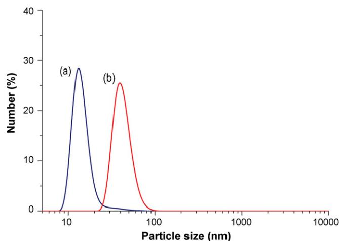
**Fig. 9.** The hydrodynamic diameter ( $D_H$ ) of (a) SPIONs (blue) and (b) commercially available MNP (red) after conjugation with OVA. (For interpretation of the references to color in this figure legend, the reader is referred to the web version of the article.)
